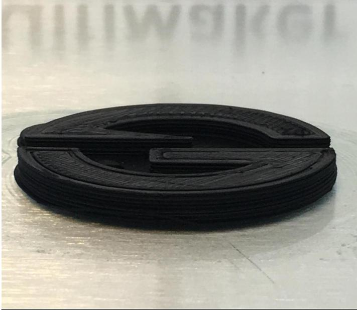
3D-printed with conductive engineering plastic (preview picture). Picture: Graphmatech AB
